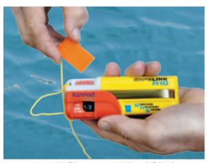
Easy activation – just slide off the orange arming tab, then pull off the red activation cap
