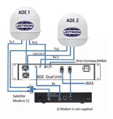
The Dual solution also gives a greater freedom in where to install the antenna. It also gives a back-up in case failure in one ADE (Above Deck Equipment).
