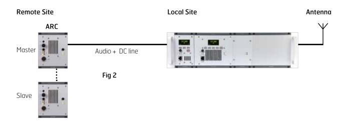
The maximum distance between ARC and radio unit is approximately 2 km, provided a high quality screened cable is used.
