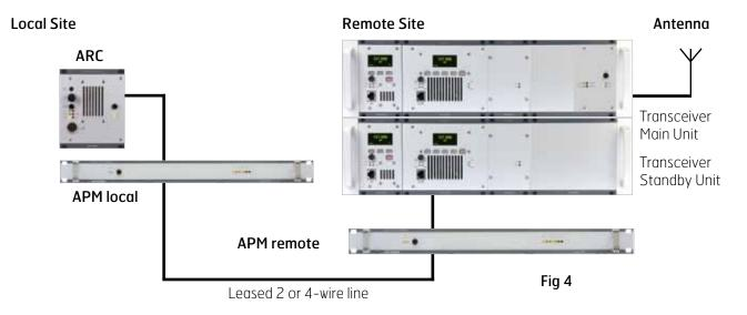
The Audio/PTT modem uses in-band tones for transfer of Squelch and PTT. Alarm (Main and Standby unit) and Main/Standby selection uses FSK data. 4 wire communication gives better audio quality and more stable communication and are recommended for challenging lines. The number of wires must be specified in the order (2 or 4 wire).
