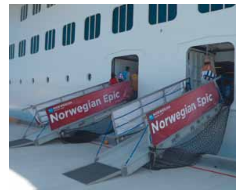
GRP-built gangways with straight and non-skid surface
