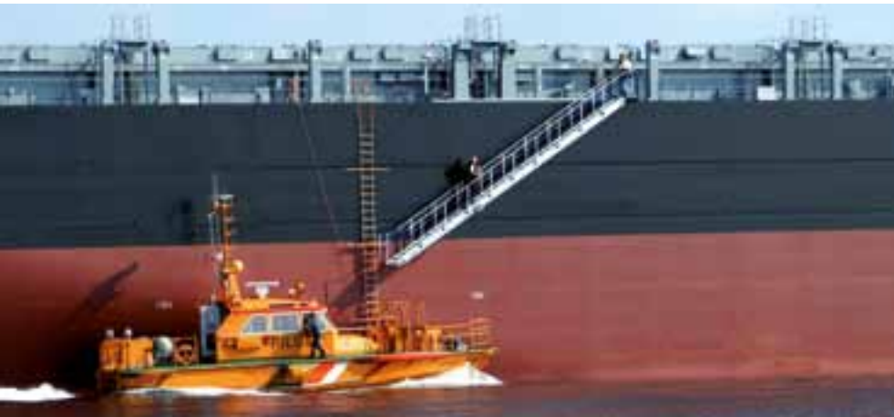
Accommodation ladder plant including pilot ladder
