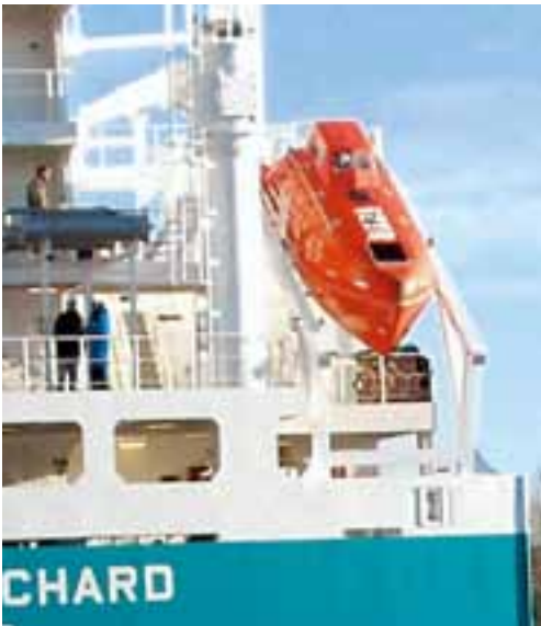
Fassmer Launching Ramp | FLR
